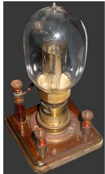
Fleming 'Oscillation Valve' 1918 (Platinum filament)
